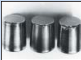
Bearing adjustment too loose
