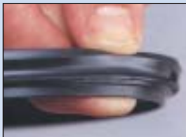
Baked from loss of lubrication
